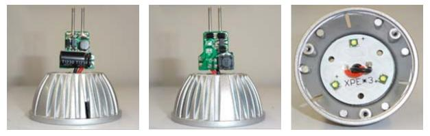
Figure 8: (a) and (b) LED Lamp and Regulation Circuits, (c) 3 LEDs in Series
