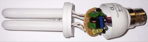
Figure 5: Dismantled CFL showing Complex Ballast Circuit
